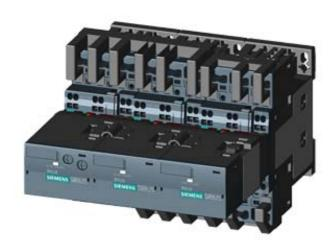
STAR-DELTA COMB. AC3, 15/18.5KW/400V AC230V, 50/60HZ, 3-POLE SZ S0, SPRING-LOADED TERMINAL ELECTR. AND MECH. INTERLOCK 3NO+3NC INTEGR.
