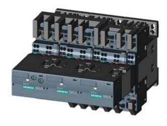
STAR-DELTA COMB. AC3, 15/18.5KW/400V AC24V, 50/60HZ, 3-POLE, SZ S0, SPRING-LOADED TERMINAL ELECTR. AND MECH. INTERLOCK 3NO+3NC INTEGR.
