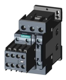
CONTACTOR, AC-3, 11KW/400V, 2NO+2NC, AC110V 50HZ, 3-POLE, SZ SO SCREW TERMINAL REMOVABLE AUX. SWITCH
