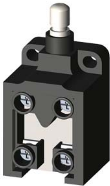
SIRIUS POSITION SWITCH; PLASTIC HOUSING OPEN TYPE 30MM 1NO/1NC SNAP- ACTION CONTACTS TEFLON PLUNGER, IP20
