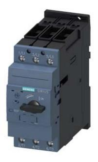
CIRCUIT BREAKER SIZE S2. FOR MOTOR PROTECTION, CLASS 20, A-RELEASE 20...25A, N-RELEASE 325A, SCREW TERMINAL, STANDARD BREAKING CAPACITY
