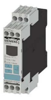
DIGITAL MONITORING RELAY FOR FAULT CURRENT MONITORING (W. CURRENT TRANSFORMER 3UL23) SETTING RANGE 0.03A TO 40A SEPARATE FOR ALARM THRESHOLD AND SWITCH-OFF VALUE SUPPLY VOLTAGE AC/DC 24 .. 240 V, 50 .. 60 HZ STARTUP AND TRIPPING DELAY 0.1 TO 20S SWITCH-OFF HYSTERESIS UP TO 50% ALARM HYSTERESIS 5% FIXED WIDTH 22.5 MM, 2 CO CONTACTS W. OR W/O ERROR LOG SCREW TERMINAL
