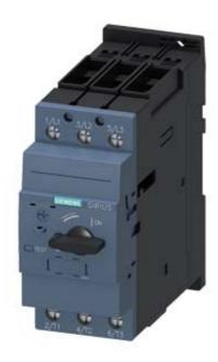
CIRCUIT BREAKER SIZE S2, FOR MOTOR PROTECTION, CLASS 10, A-RELEASE 14...20A, N-RELEASE 260A, SCREW TERMINAL, STANDARD BREAKING CAPACITY
