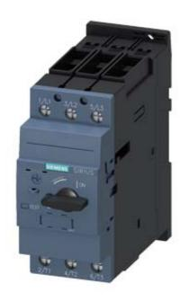
CIRCUIT BREAKER, SIZE S2, FOR MOTOR PROTECTION, CLASS 20, A-RELEASE 14...20A, N-RELEASE 260A, SCREW TERMINAL, STANDARD BREAKING CAPACITY
