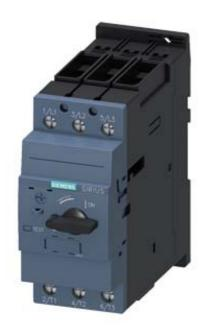
CIRCUIT BREAKER, SIZE S2, FOR MOTOR PROTECTION, CLASS 10, A-RELEASE 35...45A, N-RELEASE 650A, SCREW TERMINAL, STANDARD BREAKING CAPACITY
