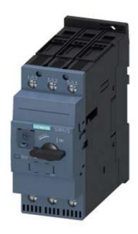
CIRCUIT BREAKER, SIZE S2, FOR MOTOR PROTECTION, CLASS 10, A-RELEASE 42...52A, N-RELEASE 741A, SCREW TERMINAL, STANDARD BREAKING CAPACITY
