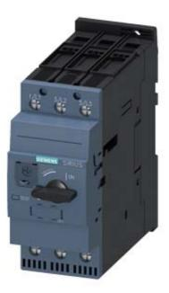
CIRCUIT BREAKER, SIZE S2, FOR MOTOR PROTECTION, CLASS 10, A-RELEASE 42...52A, N-RELEASE 741A, SCREW TERMINAL, INCREASED SWITCHING CAPACITY
