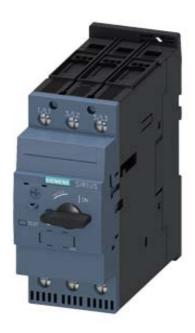
CIRCUIT BREAKER, SIZE S2, FOR MOTOR PROTECTION, CLASS 10, A-RELEASE 9.5...14A, N-RELEASE 208A, SCREW TERMINAL, INCREASED SWITCHING CAPACITY
