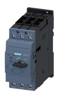
CIRCUIT BREAKER SIZE S2, FOR MOTOR PROTECTION, CLASS 20, A-REL. 22...32A, N-REL. 416A, SCREW TERMINAL, STANDARD BREAKING CAPACITY
