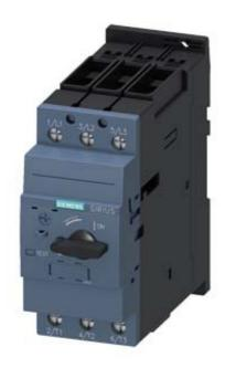
CIRCUIT BREAKER SIZE S2. FOR MOTOR PROTECTION, CLASS 10, A-REL. 22...32A, N-REL. 416A, SCREW TERMINAL, STANDARD BREAKING CAPACITY
