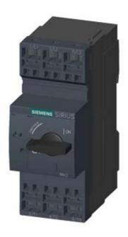
CIRCUIT-BREAKER SZ S0, FOR MOTOR PROTECTION, CLASS 10, A-REL. 9..12.5A, N-REL. 163A, SPRING-L. CONNECTION, STANDARD SW. CAPACITY
