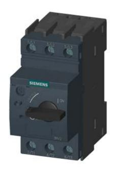
CIRCUIT-BREAKER SZ S0, FOR MOTOR PROTECTION, CLASS 10, A-REL.2.2...3.2A, N-REL. 42A SCREW CONNECTION, STANDARD SW. CAPACITY
