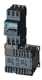
LOAD FEEDER FUSELESS REVERSING DUTY, AC 400V, SZ S00, 5,5...8A, AC 230V SPRING-LOADED CONNECTION FOR RAIL-MOUNTING, TYPE OF COORDINATION 1, IQ = 150KA 1NC (CONTACTOR)
