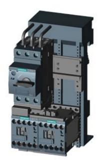
LOAD FEEDER FUSELESS REVERSING DUTY, AC 400V, SZ S00, 9. . .12.5A, AC 230V SCREW CONNECTION FOR BUSBAR SYSTEMS 60MM TYPE OF COORDINATION 1, IQ = 150KA 1NC (CONTACTOR)
