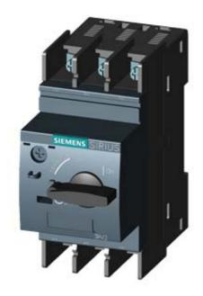
CIRCUIT-BREAKER SZ S0, FOR MOTOR PROTECTION, CLASS 10, A-RELEASE 20...25A, N-RELEASE 325A, RING CABLE LUG CONNECTION, STANDARD SW. CAPACITY,
