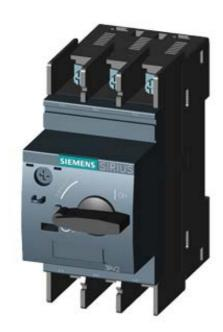
CIRCUIT-BREAKER SZ S0, FOR MOTOR PROTECTION, CLASS 10, A-RELEASE 14...20A, N-RELEASE 260A, RING CABLE LUG CONNECTION, STANDARD SW. CAPACITY,
