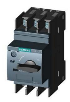
CIRCUIT-BREAKER SZ S0, FOR MOTOR PROTECTION, CLASS 10, A-RELEASE 23...28A, N-RELEASE 364A, RING CABLE LUG CONNECTION, STANDARD SW. CAPACITY,
