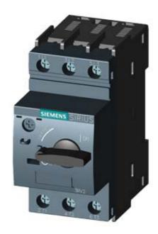
CIRCUIT-BREAKER SZ S0, FOR TRANSFORMER PROT. A-RELEASE 20...25A, N-RELEASE 400A, SCREW CONNECTION, STANDARD SW. CAPACITY
