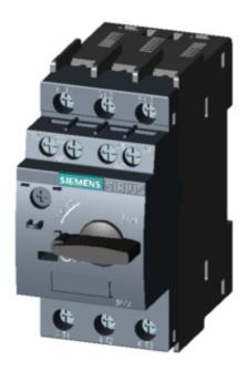
CIRCUIT-BREAKER SZ S0, FOR TRANSFORMER PROT. A-RELEASE 14...20A, N-RELEASE 325A, SCREW CONNECTION, STANDARD SW. CAPACITY W. TRANSVERSE AUX. SWITCH 1NO+1NC
