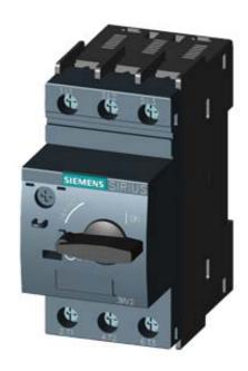
CIRCUIT-BREAKER SZ S0, FOR TRANSFORMER PROT. A-RELEASE 11...16A, N-RELEASE 286A, SCREW CONNECTION, STANDARD SW. CAPACITY
