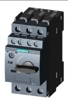
CIRCUIT-BREAKER SZ S0, FOR TRANSFORMER PROT. A-RELEASE 20...25A, N-RELEASE 400A, SCREW CONNECTION, STANDARD SW. CAPACITY W. TRANSVERSE AUX. SWITCH 1NO+1NC
