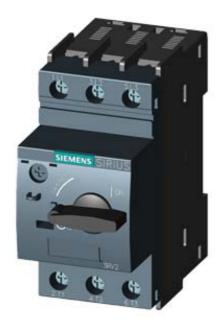
CIRCUIT-BREAKER SZ S0, FOR TRANSFORMER PROT. A-RELEASE 17...22A, N-RELEASE 364A, SCREW CONNECTION, STANDARD SW. CAPACITY
