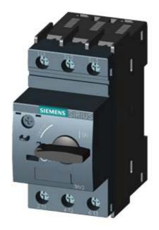
CIRCUIT-BREAKER SZ S0, FOR MOTOR PROTECTION, CLASS 10, A-RELEASE 30...36A, N-RELEASE 432A, SCREW CONNECTION, STANDARD SW. CAPACITY,
