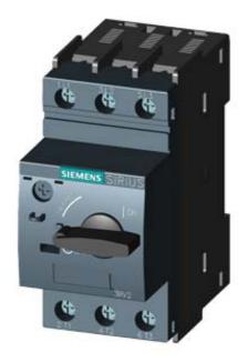
CIRCUIT-BREAKER SZ S0, FOR MOTOR PROTECTION, CLASS 10, A-RELEASE 23...28A, N-RELEASE 364A, SCREW CONNECTION, STANDARD SW. CAPACITY,
