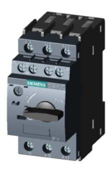
CIRCUIT-BREAKER SZ S0, FOR MOTOR PROTECTION, CLASS 10, A-RELEASE 17...22A, N-RELEASE 286A, SCREW CONNECTION, STANDARD SW. CAPACITY, W. TRANSVERSE AUX. SWITCH 1NO+1NC
