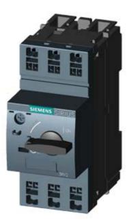
CIRCUIT-BREAKER SZ S00, FOR TRANSFORMER PROT. A-RELEASE 1.4...2A, N-RELEASE 42A, SPRING-L. CONNECTION, STANDARD SW. CAPACITY
