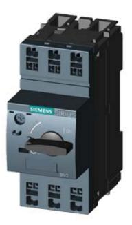
CIRCUIT-BREAKER SZ S00, FOR TRANSFORMER PROT. A-RELEASE 2.2...3.2A, N-RELEASE 65A SPRING-L. CONNECTION, STANDARD SW. CAPACITY
