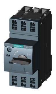
CIRCUIT-BREAKER SZ S00, FOR TRANSFORMER PROT. A-RELEASE 0.45...0.63A, N-RELEASE13A SPRING-L. CONNECTION, STANDARD SW. CAPACITY
