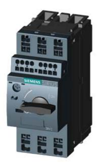
CIRCUIT-BREAKER SZ S00, FOR MOTOR PROTECTION, CLASS 10, A-RELEASE 7...10A, N-RELEASE 130A, SPRING-L. CONNECTION, STANDARD SW. CAPACITY W. TRANSVERSE AUX. SWITCH 1NO+1NC
