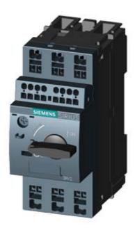
CIRCUIT-BREAKER SZ S00, FOR MOTOR PROTECTION, CLASS 10, A-RELEASE 9..12.5A, N-RELEASE 156A, SPRING-L. CONNECTION, STANDARD SW. CAPACITY W. TRANSVERSE AUX. SWITCH 1NO+1NC
