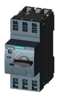
CIRCUIT-BREAKER SZ S00, FOR MOTOR PROTECTION, CLASS 10, A-RELEASE 4.5...6.3A, N-RELEASE 82A SPRING-L. CONNECTION, STANDARD SW. CAPACITY
