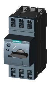
CIRCUIT-BREAKER SZ S00, FOR MOTOR PROTECTION, CLASS 10, A-RELEASE 7...10A, N-RELEASE 130A, SPRING-L. CONNECTION, STANDARD SW. CAPACITY
