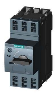
CIRCUIT-BREAKER SZ S00, FOR MOTOR PROTECTION, CLASS 10, A-RELEASE 3.5...5A, N-RELEASE 65A, SPRING-L. CONNECTION, STANDARD SW. CAPACITY
