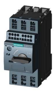
CIRCUIT-BREAKER SZ S00, FOR MOTOR PROTECTION, CLASS 10, A-RELEASE 5.5...8A, N-RELEASE 104A, SPRING-L. CONNECTION, STANDARD SW. CAPACITY W. TRANSVERSE AUX. SWITCH 1NO+1NC
