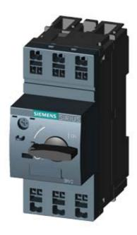
CIRCUIT-BREAKER SZ S00, FOR MOTOR PROTECTION, CLASS 10, A-RELEASE 5.5...8A, N-RELEASE 104A, SPRING-L. CONNECTION, STANDARD SW. CAPACITY
