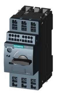
CIRCUIT-BREAKER SZ S00, FOR MOTOR PROTECTION, CLASS 10, A-REL.1.8...2.5A, N-RELEASE 33A, SPRING-L. CONNECTION, STANDARD SW. CAPACITY W. TRANSVERSE AUX. SWITCH 1NO+1NC
