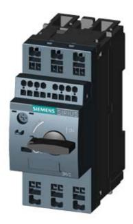
CIRCUIT-BREAKER SZ S00, FOR MOTOR PROTECTION, CLASS 10, A-RELEASE2.2...3.2A, N-RELEASE 42A, SPRING-L. CONNECTION, STANDARD SW. CAPACITY W. TRANSVERSE AUX. SWITCH 1NO+1NC
