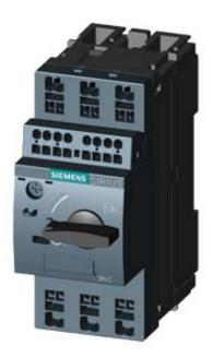
CIRCUIT-BREAKER SZ S00, FOR MOTOR PROTECTION, CLASS 10, A-REL. 0.7...1A, N-RELEASE 13A, SPRING-L. CONNECTION STANDARD SW. CAPACITY W. TRANSVERSE AUX. SWITCH 1NO+1NC
