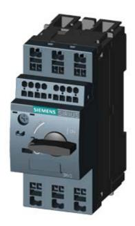
CIRCUIT-BREAKER SZ S00, FOR MOTOR PROTECTION, CLASS 10, A-REL. 0.9...1.25A, N-RELEASE16A, SPRING-L. CONNECTION STANDARD SW. CAPACITY W. TRANSVERSE AUX. SWITCH 1NO+1NC
