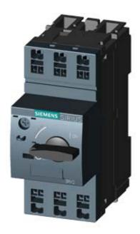
CIRCUIT-BREAKER SZ S00, FOR MOTOR PROTECTION, CLASS 10, A-REL. 0.9...1.25A, N-RELEASE16A, SPRING-L. CONNECTION STANDARD SW. CAPACITY
