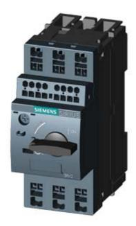
CIRCUIT-BREAKER SZ S00, FOR MOTOR PROTECTION, CLASS 10, A-REL. 0.22...0.32A, N-RELEASE4.2A SPRING-L. CONNECTION STANDARD SW. CAPACITY W. TRANSVERSE AUX. SWITCH 1NO+1NC
