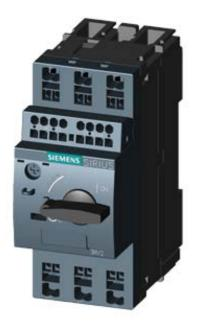
CIRCUIT-BREAKER SZ S00, FOR MOTOR PROTECTION, CLASS 10, A-RELEASE 0.11...0.16A, N-RELEASE2.1A SPRING-L. CONNECTION STANDARD SW. CAPACITY W. TRANSVERSE AUX. SWITCH 1NO+1NC
