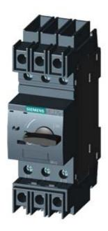
CIRCUIT-BREAKER SZ S00, FOR TRANSFORMER PROTECTION, WITH APPROBATION CIRCUIT-BREAKER UL 489. CSA C22.2 NO.5-02. A-RELEASE 10 A, N-RELEASE 208 A, SCREW CONNECTION, STANDARD SW. CAPACITY
