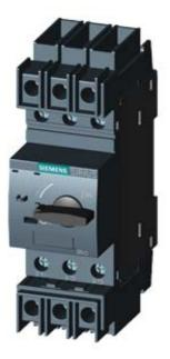
CIRCUIT-BREAKER SZ S00, FOR TRANSFORMER PROTECTION, WITH APPROBATION CIRCUIT-BREAKER UL 489. CSA C22.2 NO.5-02. A-RELEASE 8 A, N-RELEASE 163 A, SCREW CONNECTION, STANDARD SW. CAPACITY
