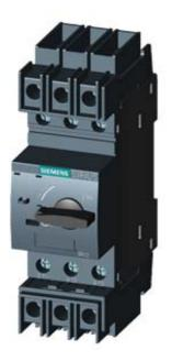
CIRCUIT-BREAKER SZ S00, FOR TRANSFORMER PROTECTION, WITH APPROBATION CIRCUIT-BREAKER UL 489. CSA C22.2 NO.5-02. A-RELEASE 5 A, N-RELEASE 104 A, SCREW CONNECTION, STANDARD SW. CAPACITY
