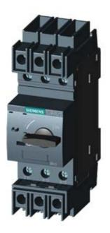
CIRCUIT-BREAKER SZ S00, FOR TRANSFORMER PROTECTION, WITH APPROBATION CIRCUIT-BREAKER UL 489. CSA C22.2 NO.5-02. A-RELEASE 3.2 A, N-RELEASE 65 A, SCREW CONNECTION, STANDARD SW. CAPACITY
